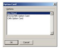
Selecting the appropriate card will add an icon to tree shown in the left-hand pane of the window. This icon will in turn contain icons for the additional port or ports that are made available by the card. The example below shows a G3 with a serial expansion card installed...
