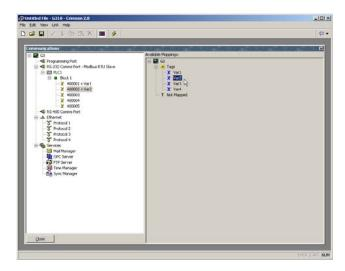
In the example above, tags *Var1* and *Var2* have been mapped to registers **400001** through **400002**. The direction of the arrows indicates that the G3 provides these values into the PLC (So the PLC can only read them).
