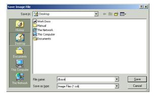
The Save Image command will create a MonicoView database image file with a CDI extension. It will also save a copy of the current G3 firmware to a file with a BIN extension. The image file must be given the name DBASE.CDI, and both it and the BIN file must be placed in the root directory of a CompactFlash card. To update a G3 panel, power down the
