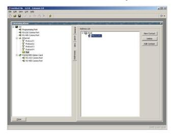
An unlimited number of address book entries can be added, edited or deleted using the buttons in the right-hand pane. Each entry can refer to one or more email recipients from any of the transports enabled by the database. Recipients for multiple transports can be included in the same entry. The dialog used to define the properties of each recipient is shown below...
