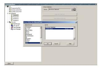
The properties available on HMI1 are the server's OPC and Ethernet settings. The *IP Address* and *TCP Port* should match the server's. The *Browse* button provides access to a dialog box where the server database should be identified. Using this method, MonicoView knows the tags available in the server unit. The tag list is pulled from the server database so it can be available when mapping new tags in the client.
