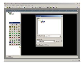
The tag is ready to be inserted. Just click, hold and drag the mouse cursor across the screen to insert the tag. Repeat the same operation for all the tags you whish to display in that page.
