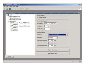
For most protocols, this will produce higher performance, as it will allow simultaneous communications with the two devices. It will, however, consume two of the four protocols, limiting your ability to connect via additional protocols in complex applications. Your second option is therefore to use a single protocol configured as a Modbus TCP/IP Master, but to add a further device so that both slaves are accessed via the same driver...
