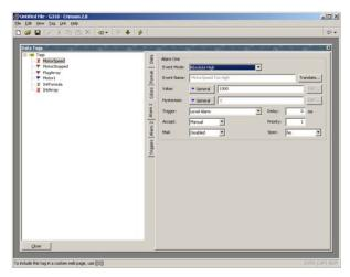
• The *Event Mode* property is used to indicate the logic that will be used to decide whether the alarm should activate. The tables below list the available modes.
