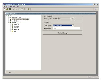
The device properties are a subset of those provided for dial-in connections. SMS support is always enabled with this driver, but once again, note that in order for SMS messaging to operate properly, you will also have to enable the SMS Transport using the Mail icon in the Communications window.
