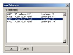
The dialog lists the models supported by the current version of the software, providing a description of each terminal and the dimensions of its display. Selecting a terminal will create a blank database, and reconfigure MonicoView to work with that specific model.
