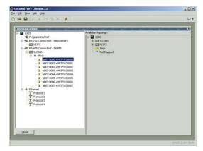
To move data between two master devices, simply select one of the devices, and create a Gateway Block for that device. You can then add references to the other device's registers just as you would when exposing data on a slave protocol. Again, C2 will automatically read
