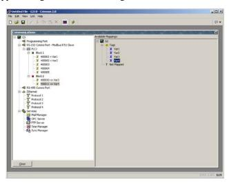
Note the color of the block is red telling you the PLC can write data in any registers linked to this block. The arrows also indicate that the PLC can also read data from the block, so this block has a Read/Write access.
