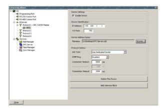
When creating data tags, the server tags will be accessible via the mapping button. A client tag can be linked to one of the server's tags. Once used in the database, reading or writing this tag will access the server with the appropriate command and action with no further programming necessary. If the server tag is related to a PLC, changing the client tag will impact on the server, which in turn will reflect the change in the PLC.
