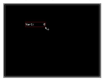
To be able to change the data in the PLC from the G310 HMI screen, for example *Var2*, double click *Var2* in the User Interface to access the primitive properties and change *Data Entry* to yes on the Properties Tab as shown below.
