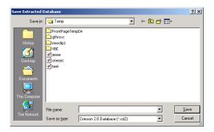
Note that if you lose your database file and you do not have upload support enabled, you will not be able to reconstruct your file without starting from scratch. To extract a database from a panel, use the Link-Extract command. This command will upload the database, and then prompt you for a name under which to save the file. The file will then be opened for editing.
