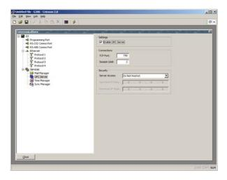
The *Security* properties are used to restrict OPC server access to hosts whose IP address matches the mask and data indicated. All access may be restricted, or the filter may be used to restrict only attempts to write data in the server. The filter works in the following way:
