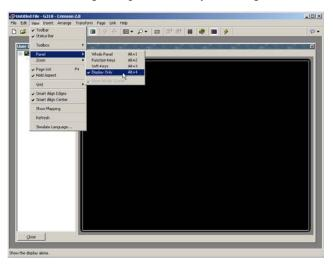
Click on the black screen so the Drawing toolbox appears. To insert the tags on the screen simply click the tag icon in the drawing toolbox. In the Select Tag dialog box, select one of the tags and click ok.
