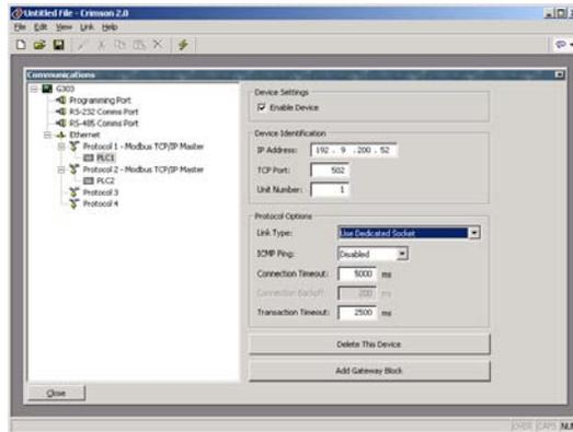
For most protocols, this will produce higher performance, as it will allow simultaneous communications with the two devices. It will, however, consume two of the four protocols, limiting your ability to connect via additional protocols in complex applications. Your second option is therefore to use a single protocol configured as a Modbus TCP/IP Master, but to add a further device so that both slaves are accessed via the same driver...
