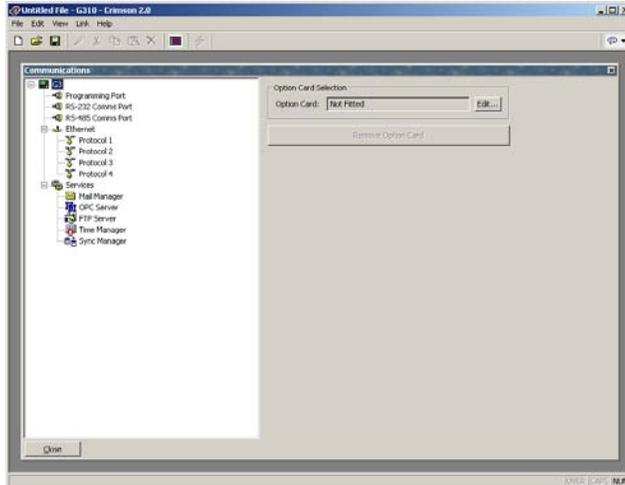
Select the communication port your PLC should be connected to (in this example, the RS232 Comms Port) and click the Edit button in the driver selection area to choose a protocol. In this example, Allen Bradley DF1 Master has been selected as the protocol.
