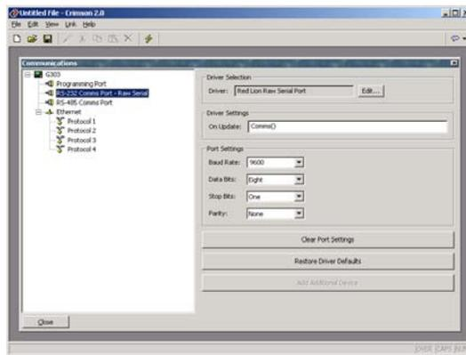
The port’s Baud rate and other byte format parameters should be configured to indicate the required communications settings, and the On Update property should be set to specify the program that will be performing the communication. This program will be called continually by the port’s communications task.
