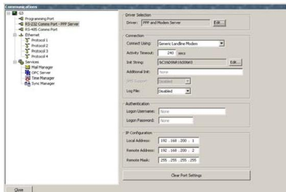
For a PPP and modem client configuration, the G3 will most likely connect to the Internet using an Internet access provider. The IP address to enter in your web browser is therefore the one provided by this service. For this reason, you will most likely require a fixed IP address to be able to access the G3 web server.
