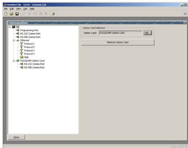
The additional ports can be configured by following the instructions supplied in the previous chapter. Note that the drivers available for a port will depend on the connection type it supports. For example, the CANOpen expansion card shows a port that will only support drivers designed for the CAN communication standard.
