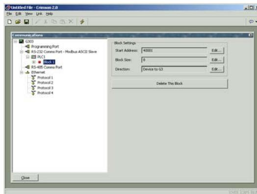
In the example above, we have configured the Start Address to 40001 to indicate that this is where we want the block to begin. We have also configured the Block Size to eight so as to allocate one Modbus register for each tag we want to expose. Finally, we have configured the
