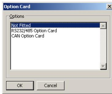
Selecting the appropriate card will add an icon to tree shown in the left-hand pane of the window. This icon will in turn contain icons for the additional port or ports that are made available by the card. The example below shows a G3 with a serial expansion card installed...
