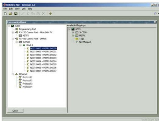
To move data between two master devices, simply select one of the devices, and create a Gateway Block for that device. You can then add references to the other device's registers just as you would when exposing data on a slave protocol. Again, C2 will automatically read
