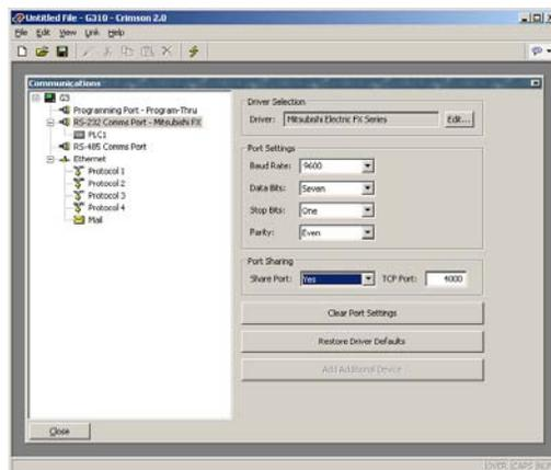
If you leave the port setting at zero, a number of 4000 plus the logical index of the port will be used. (To obtain the logical index of the port, count the port’s position in the list, noting that the programming port is always logical port 1.) You may use any number that is not already used by another TCP/IP protocol. If you are stuck for ideas, we recommend numbers between 4000 and 4099.
