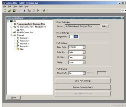
Note that the Baud rate and other port settings do not have to be the same as those for the port which we are sharing, unless the unit being programmed is a PAX meter. In that case, the PAX and the G3 port **MUST** be set for 9600 8 N 1. In the configuration shown above, data to and from the programming software is sent at a higher Baud rate than the data to and from the PLC, with the G3 doing the appropriate buffering and conversion.
