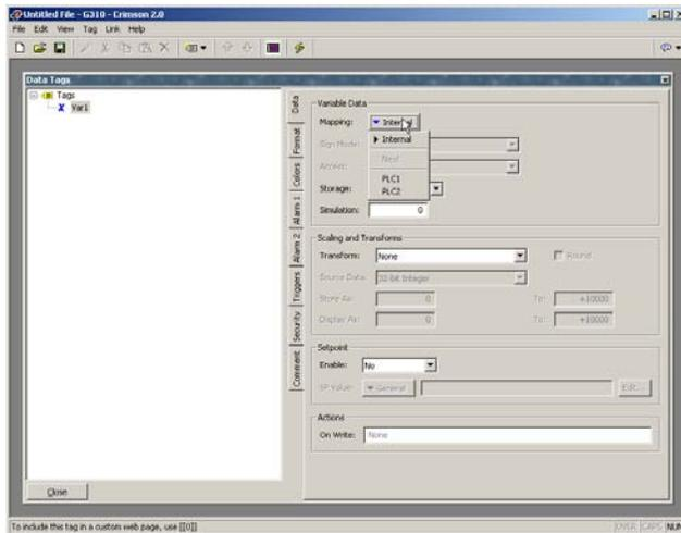
When you select the device (Here *PLC1*), a dialog box prompts you to select the register address to access in that device. Since the protocol selected was Allen Bradley DF1, the addresses available here are native Allen Bradley registers. Select for example the prefix **N** for integer and the address **0007 : 0001**. *Var1* will thus be the same as **N7:1** in the PLC.
