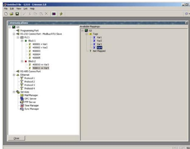
Note the color of the block is red telling you the PLC can write data in any registers linked to this block. The arrows also indicate that the PLC can also read data from the block, so this block has a Read/Write access.
