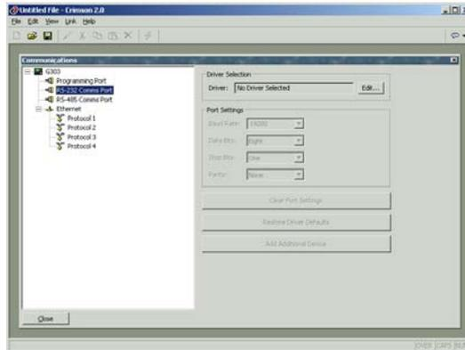
As can be seen, the Communications window lists the unit's available ports in the form of a tree structure. G3 panels have three primary serial ports, with the option to add a further two ports in the form of an expansion card. They also provide a single Ethernet port that is capable of running four communications protocols simultaneously.
