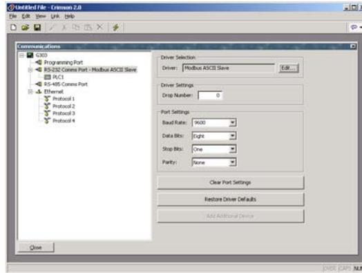
Note that a single device has been automatically created for the protocol. In the case of master protocols, this represents the remote device that the G3 will access. In this case, though, the device represents the Modbus slave that the G3 will itself embody. This means that only a single device is required, and that things such as the station number to which the G3 will respond are normally configured via the port settings rather than those of the device.
